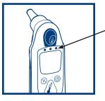
Refer to the display of your device. If three dots are visible above the display, the device must be checked for calibration every 52 weeks.
