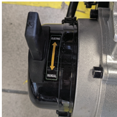
Figure 1 – Electric / Manual mode switch
