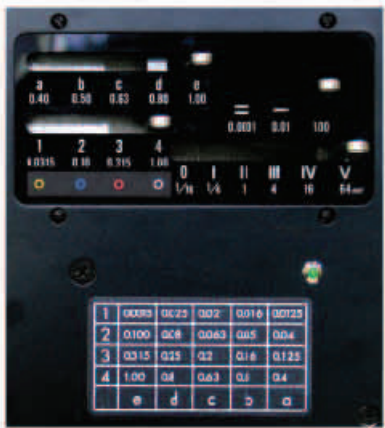
The diaphragms, the neutral density filter combination table and control levers
